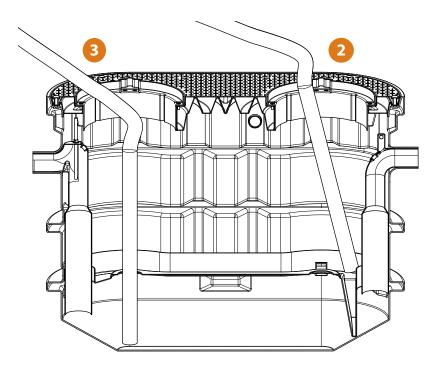
Begin by pumping grease from upper chamber, until you can see the entire horizontal baffle.
